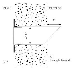
In case of fixed installation, air discharged from rear hose has been extracted from the room where the appliance is installed.
